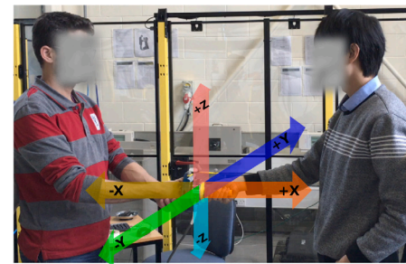
Fig. 8. human-human demonstration: two human operators holding a common object. The human operator on the right guides the demonstration by moving in each principal direction, in a random order.
