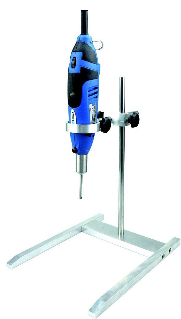
Picture 1: Tissue homogenizer similar to the one used for homogenization of organs
