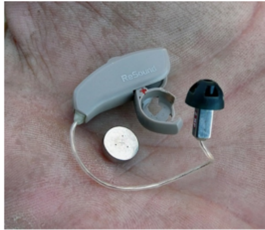
Figure 2.7. A modern behind the ear hearing aid with a minicell battery
