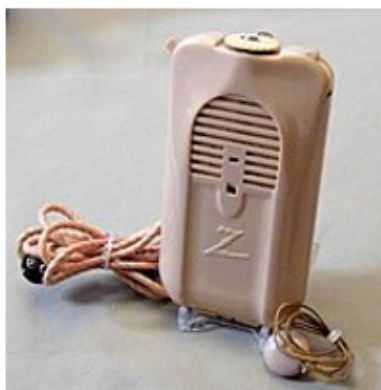
Figure 2.1 Vacuum tube hearing aid, circa 1944
