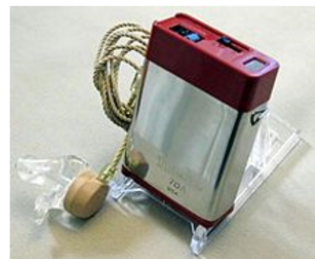
Figure 2.2 Transistor body-worn hearing aid
