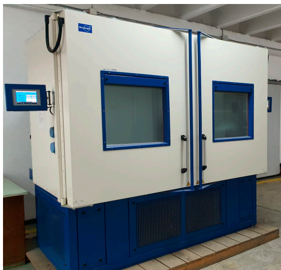
Figure 4. Double climate chamber in the work.
