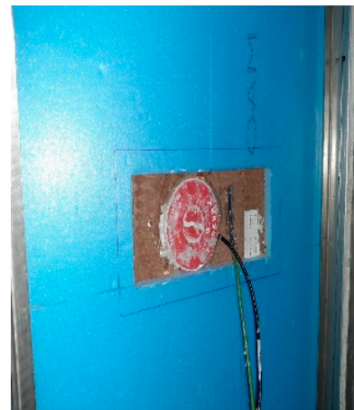
Climate chamber no. 2—cold face Temperature sensor and thermal heat flow sensor
