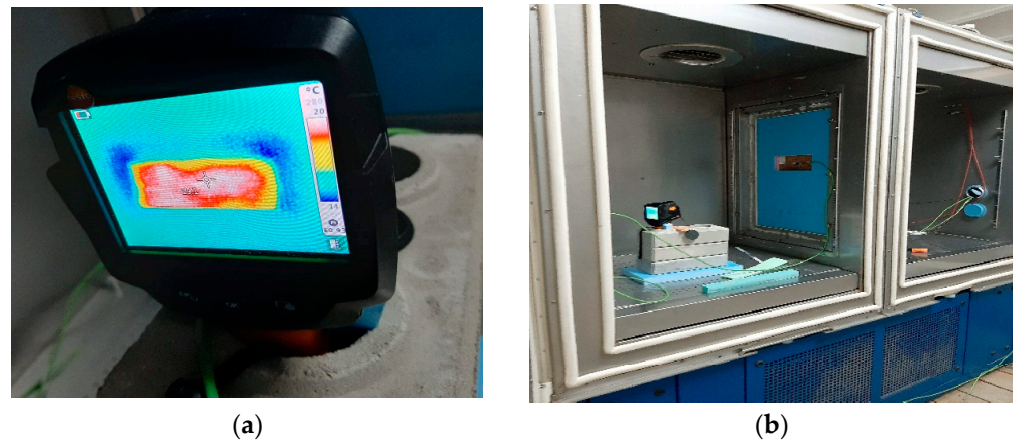
Figure 7. Thermographic test preparation in a double climate chamber. (a) Thermal image of sample no. 1; (b) Double climate chamber—test preparation.
