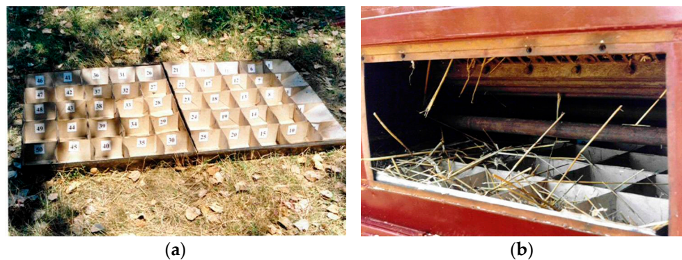
Figure 2. Block of collecting boxes. (a) Before being mounted under the threshing apparatus. (b) Mounted under the threshing apparatus.
