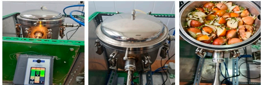
Figure 8. The experimental operation for the ultrasonic extraction mode.
