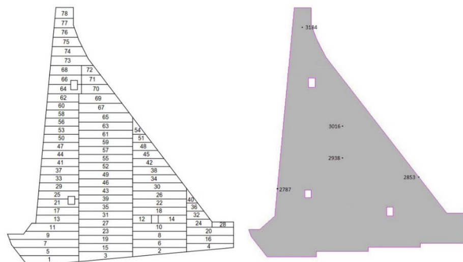
Figure 8. Distinctive control nodes of the model in the mid-plane of the monolith.
