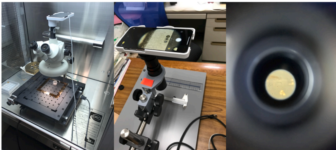
Fig. 17. Adapting the LabCam ® and iPhone Pro Max 12 into the ISAS CLOXS system. Left : Clean bench set up to start single-operator imaging and analysis. Note the LabCam ® mount, and 50 mm traverse motorised xy stage, 100 mm traverse stage and joystick controls. Centre : Hozon and LabCam ® mounted with iPhone Pro Max 12 for calibration. Right : Looking remotely ‘down the hole’ of the iPhone Pro Max 12 at a magnified block particle fragment in the aerogel.
