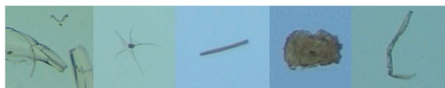
Fig. 6. Examples of Tanpopo surface objects. From left to right, aerogel fragment, sputter, bar, block and fibre.
