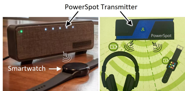
FIGURE 26. Far-field RF wireless charging system for smartwatches [144], [145].
