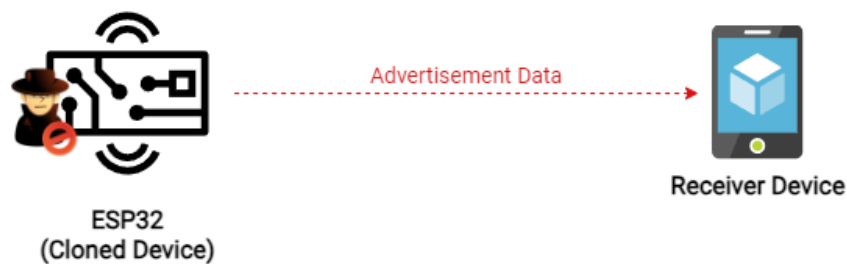
Figure 4.6: Beacon cloning architecture.
