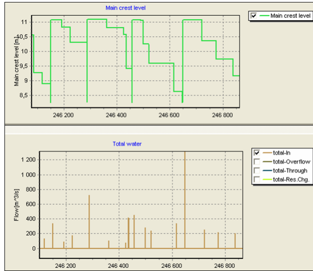
Figure 4: Compared evolution of the main crest level and the flow in the reservoir
