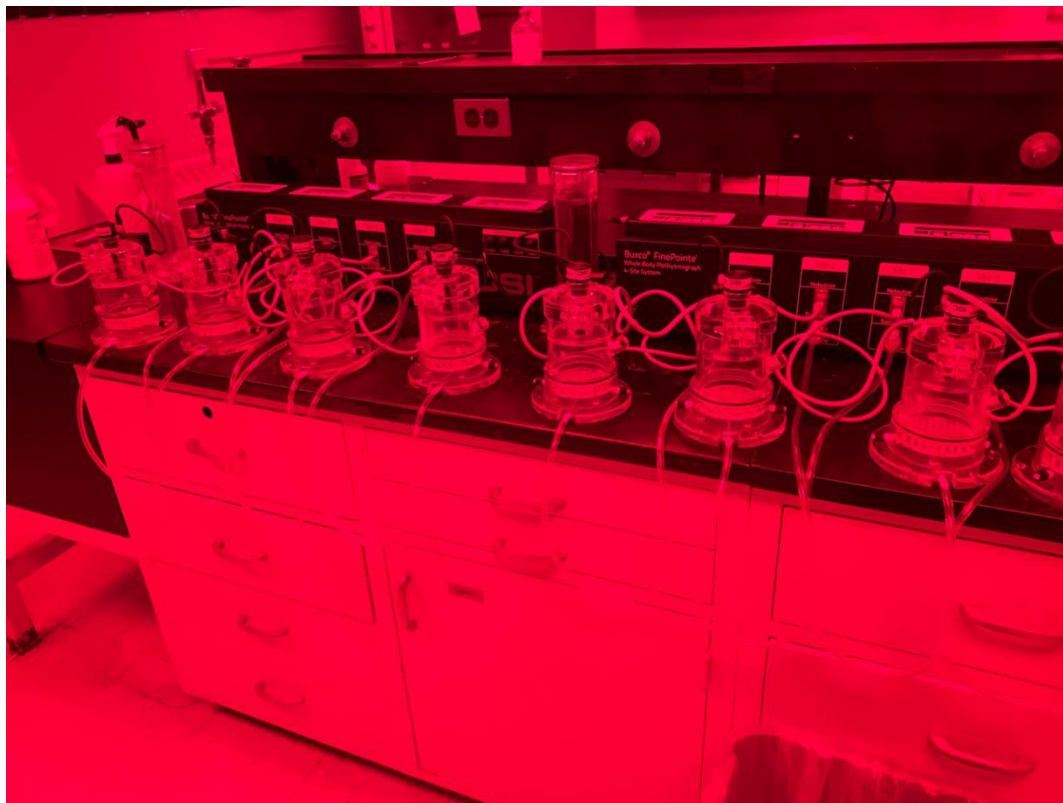
Figure 4.1: Whole-Body Plethysmography Chambers under 660 nm Lighting Conditions.
