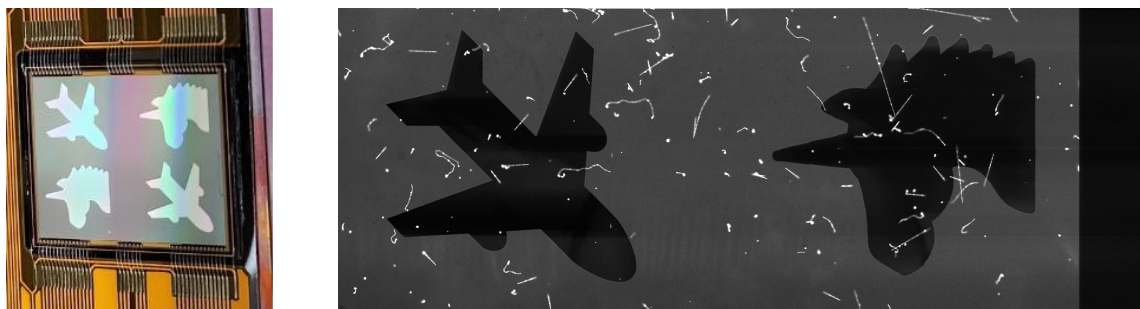
Figure 12. Oscura prototype skipper-CCD with an aluminum shield to probe the background light suppression potential of a 50 nm metal layer. (Left) Picture of the sensor with an aluminum plane- and unicorn-shaped layer on top of each quadrant. (Right) Image acquired using the upper half of the Oscura skipper-CCD after 30 minutes exposure.
