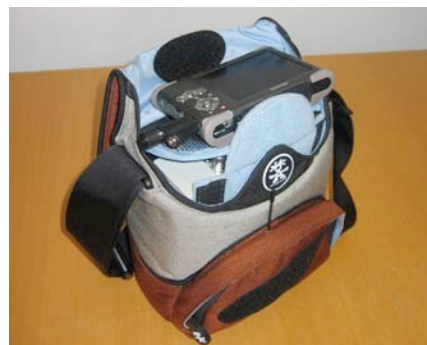
Figure 11. Our most recent version of the field laboratory weighing only 2 kg and measuring just 18x14x25 cm - containing video and audio receivers, Picture-in-Picture unit, hard disk recorder, and battery.
