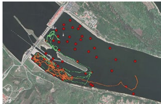
Figure 10. Movement of the one sterlet (orange line) and one vimba bream (green line) in the area under Iron Gate II dam. Red dots are location of acoustic receivers.
