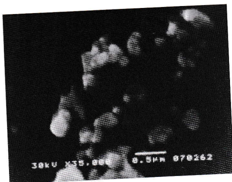
Figure 3. SEM micrograph of powder mixture of BIT and BT
