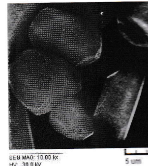
Figure 3. The microstructure of sintered sample
