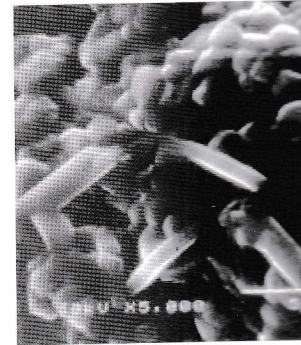
Figure 5. SEM micrograph of BBT powder sintered at 1100^\circ\text{C}
