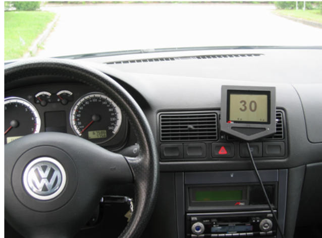
Display and loudspeaker placed in air nozzle
