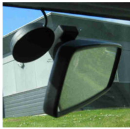
GPS Antenna placed behind the rear-view mirror
