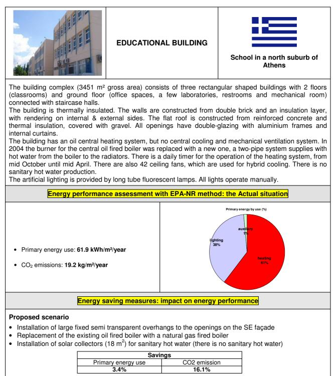
Installing external shadings results to an increase of heating energy consumption, on the other hand thermal comfort during cooling period is improved. Installation of solar collectors for DHW is attractive. These two measures increase the building comfort but do not reduce energy consumption.
