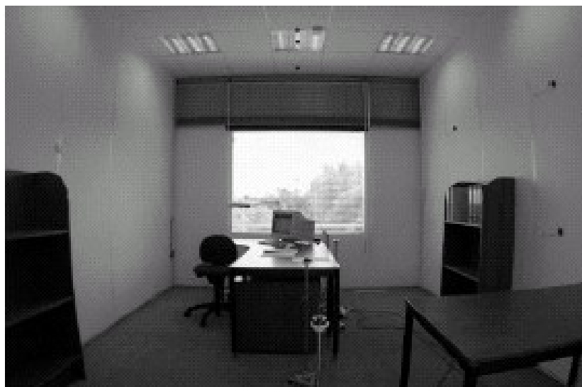
Figure 4 Interior picture of Test Room showing the window configuration (small window with a sill height of 0.8 m above the floor), arrangement of furniture for user acceptance studies and exterior obstruction.
