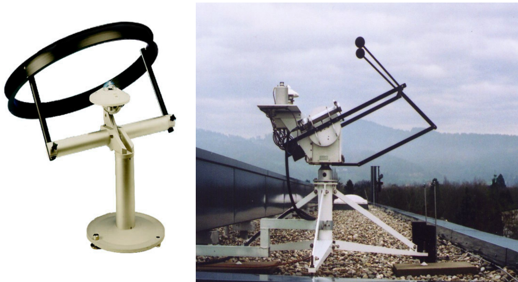
Figure 9 Picture showing the diffuse irradiance sensor screened from direct sunlight by standard shade ring (Kipp & Zonen) or by a sun-tracking ball.
