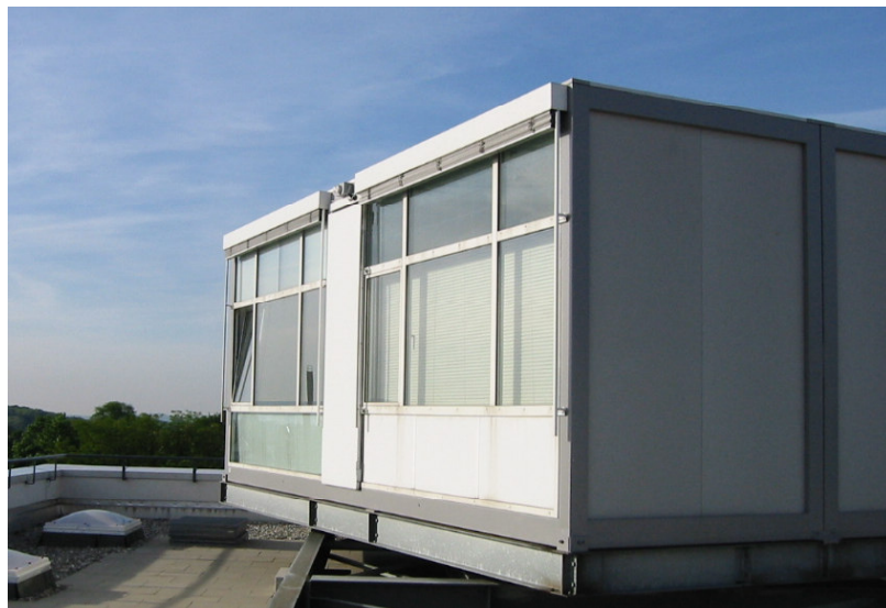
Figure 6: Picture of the Daylight Laboratory of the ISE Institute showing the two experimental rooms, which located on the roof of the building and are fully rotatable without restrictions.
