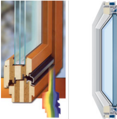
Figure 31b. Insulated frame.
