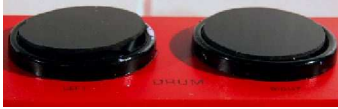
Figure 6: The hitting exciter is implemented with two drum pads. Inside each drum pad there is a pressure sensor, which picks up the force applied by the user.
