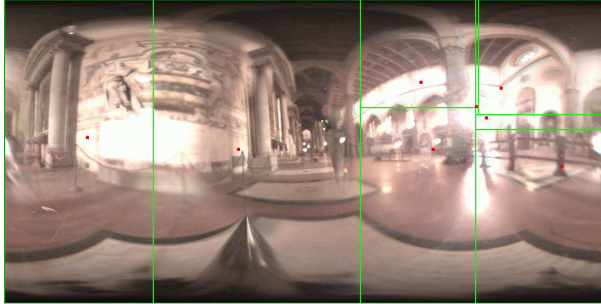
Fig. 1. Result from running the Median Cut approximation technique using 8 directional sources on Galileo’s Tomb light probe. The light probe is obtained from [10]. Each rectangular region contains a red dot. This red dot marks the chosen direction for a particular directional source, and all the combined radiance from the region has been transferred to this particular source direction.
