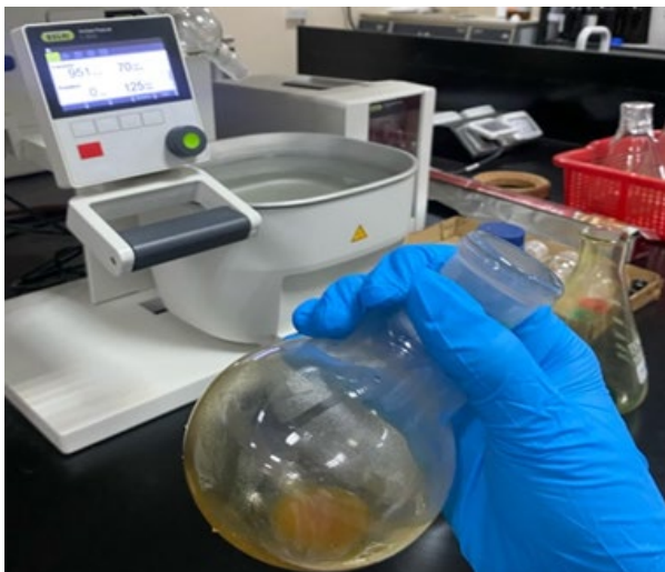
Figure 9. Evaporation Process of Methanol by Rotary Evaporator
