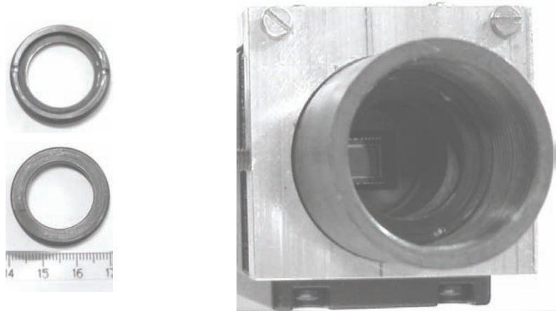
Figure H-11 Left, the lower lock nut. Right, the lower lock nut placed in the optical frame.
