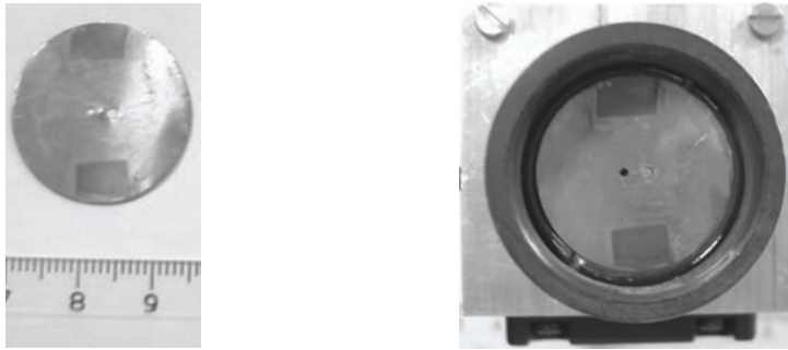
Figure H-7 Left, the pinhole optic. Right, the pinhole optic placed in the optical frame. The diameter of the left hole is 1 mm where the diameter of the right hole is 1,5 mm.
