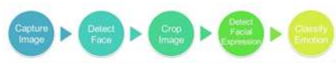
Fig 11: Emotion detection flow chart
