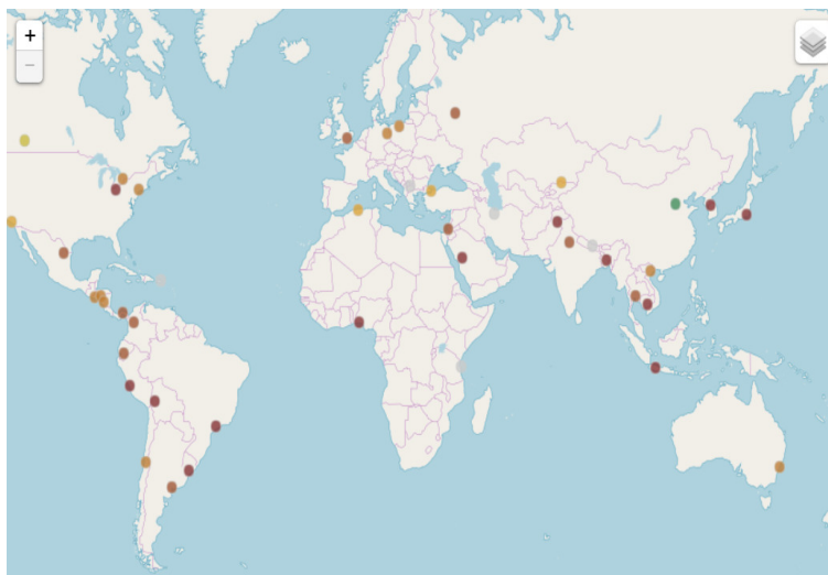
Figure 3.4: RIPE Atlas Probe Locations. The colours represent the latency associated with each DNS query response when this RIPE Atlas image was collected in our 2018 measurement study: red = high, amber = medium, green = low, grey = no data. The latency times are also summarised in Table 3.3 under the column labelled Latency.
