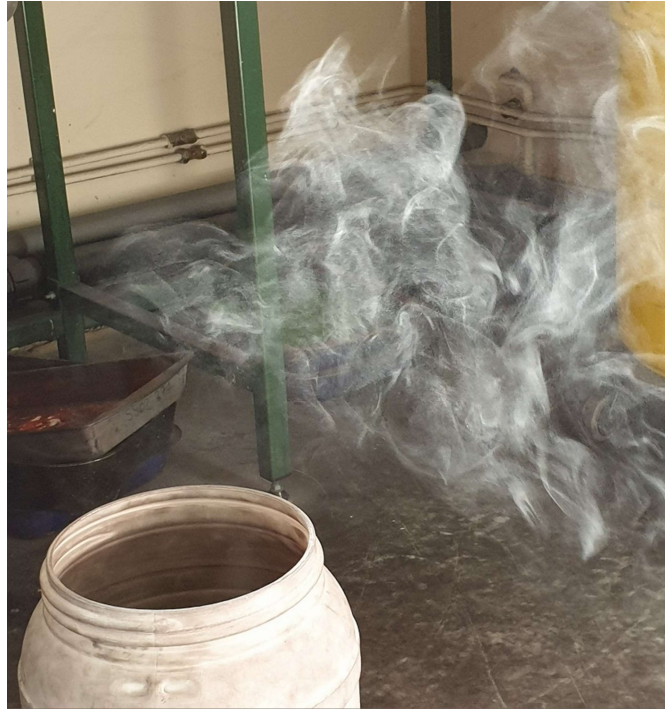
Figure 7.2: Photo demonstrating the high amount of fine material in later batches of sand. This behaviour was not observed in early batches of BL60.
