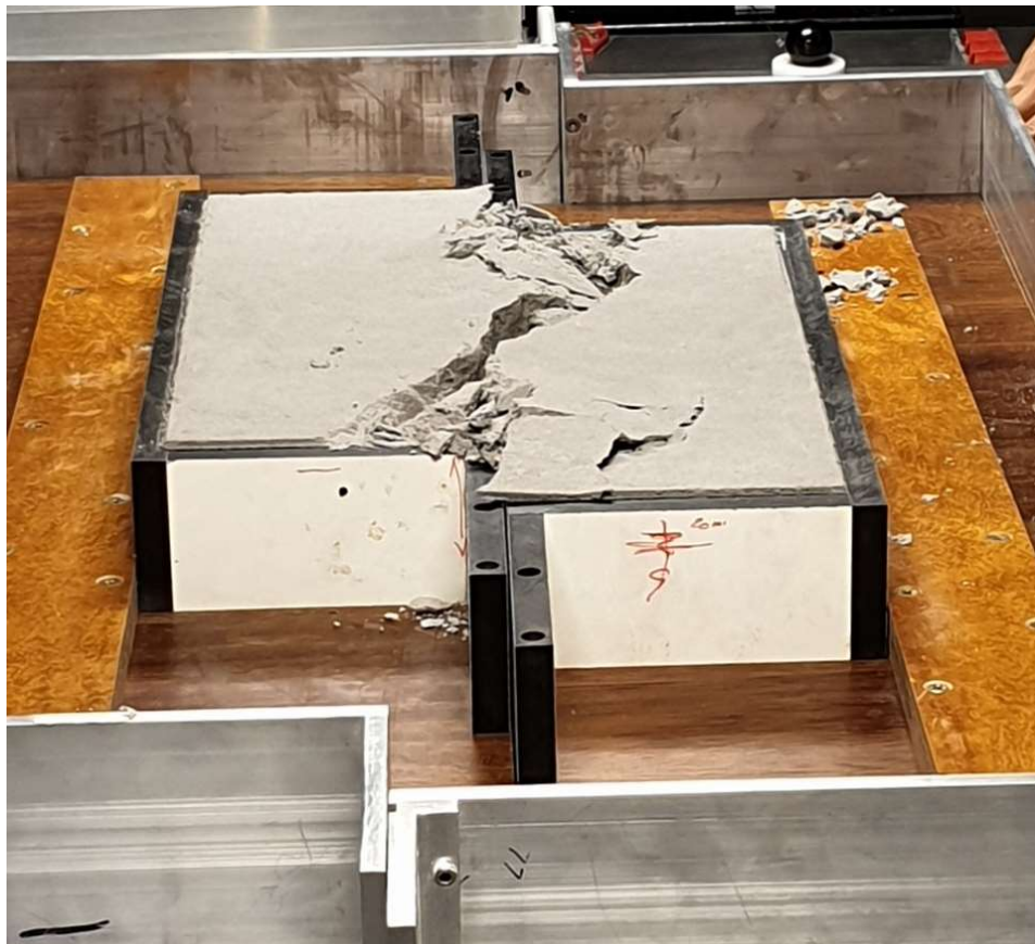
Figure 7.10: Testing of the new granular materials by shearing the ‘sandpack’. Of note is the capability to sustain open fractures as the granular material has cohesion.
