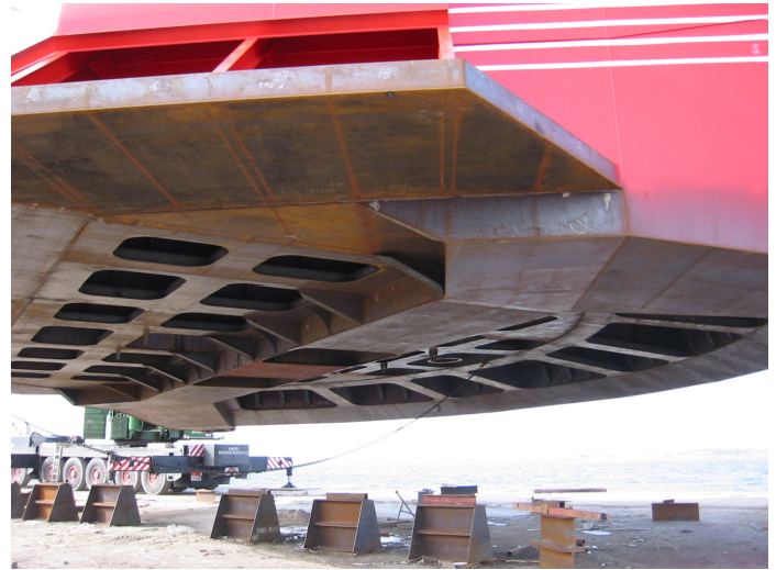
Fig. 3. WD prototype seen from beneath at launch in March 2003. The open air-chambers are used to control the floating level.
