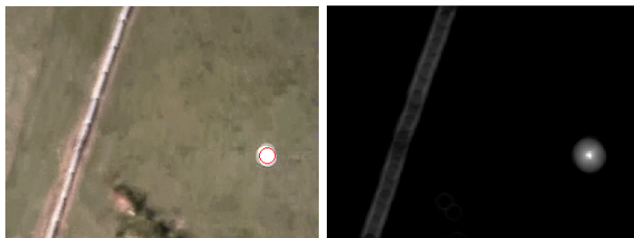
Figure 3. Left: Input to the Hough transform with the located load indicated by a circle. Right: Output of the Hough transform.
