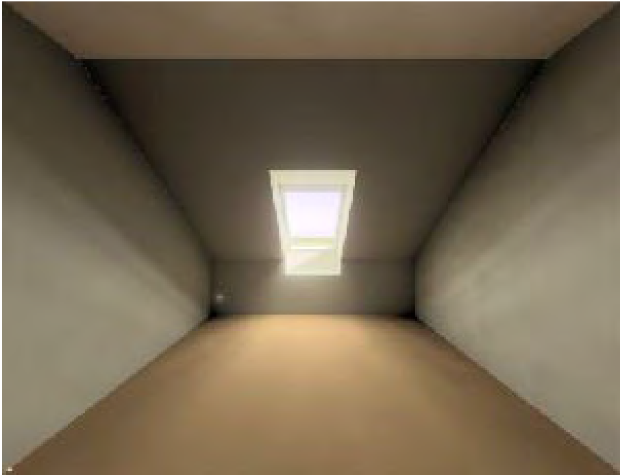
Figure 65. Radiance pcond rendition for North facing roof window in May at 10:00 hours.
