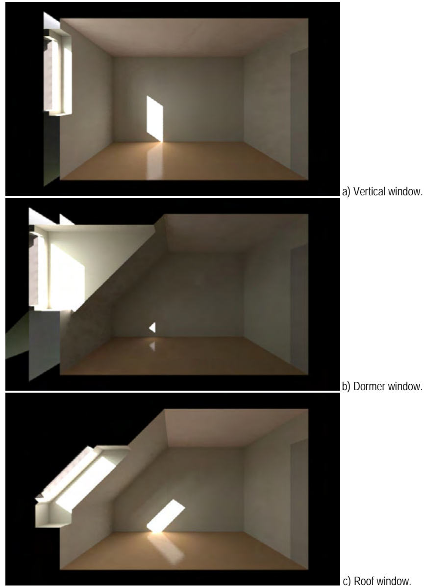
Figure 2. Rendering showing a longitudinal section-perspective of the three rooms modelled in Radiance.
