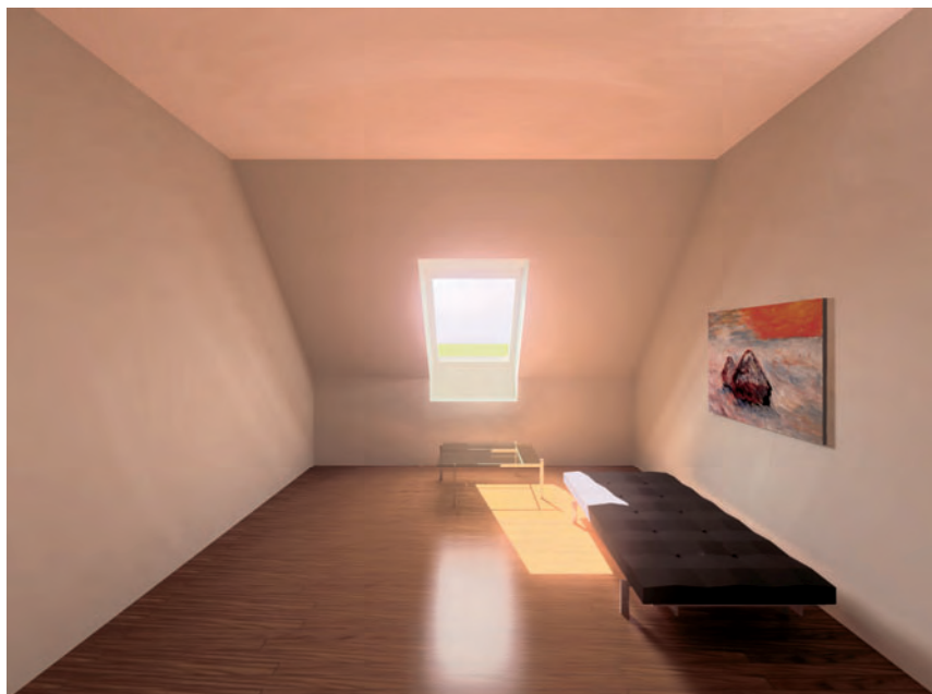
Figure 95. Radiancy images of the three rooms seen from a viewpoint in the symmetry line. The high luminance of the windows seem to be more critical with the vertical and the dormer window than with the roof window, mainly because of the higher general luminance level under the roof window.
