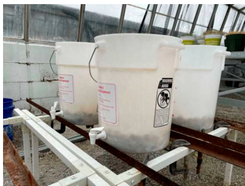
Fig. 2. Beverage dispensers with spigots filled with 10 cm (3.94 inches) of gravel used for subsurface irrigation of creeping bentgrass grown in sand-based lysimeters with nanobubble-oxygenated irrigation water.
