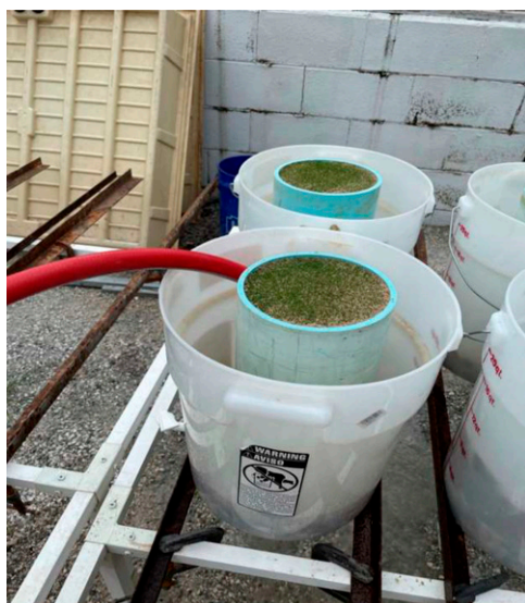
Fig. 3. Nanobubble-oxygenated irrigation water being applied directly from the nanobubble generator to the subsurface irrigation beverage dispenser (through the red hose, center left) to investigate the effects of nanobubble-oxygenated irrigation water on creeping bentgrass grown in sand-based lysimeters.
