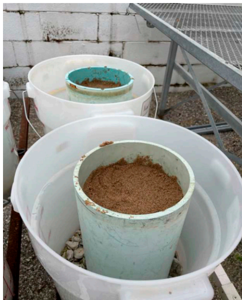
Fig. 1. An example of a polyvinyl chloride lysimeter packed with 20 cm (7.87 inches) of sand placed on 10 cm (3.94 inches) of gravel within a beverage-dispensing bucket to investigate the effect of subsurface nanobubble-oxygenated irrigation water on creeping bentgrass growth.
