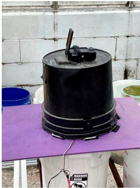
Fig. 4. Modified lightbox used to capture images digitally analyzed for green turfgrass coverage and the dark green color index of creeping bentgrass grown in sand-based lysimeters.
