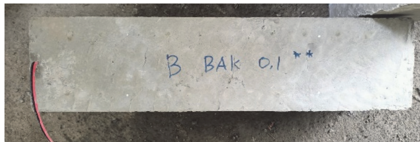
Figure 6: Example of a specimen before the corrosion acceleration process.
