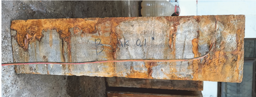
Figure 9: Example of beam specimen after the corrosion acceleration process.
