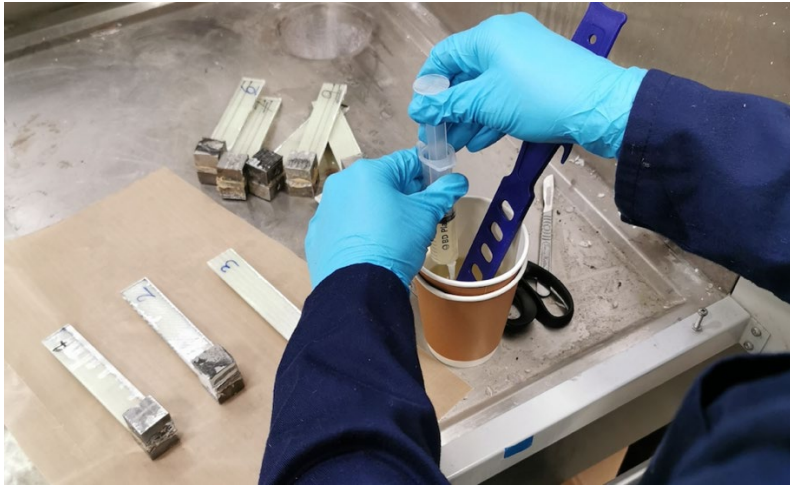
Fig. 1. Preparation of injection repair process
