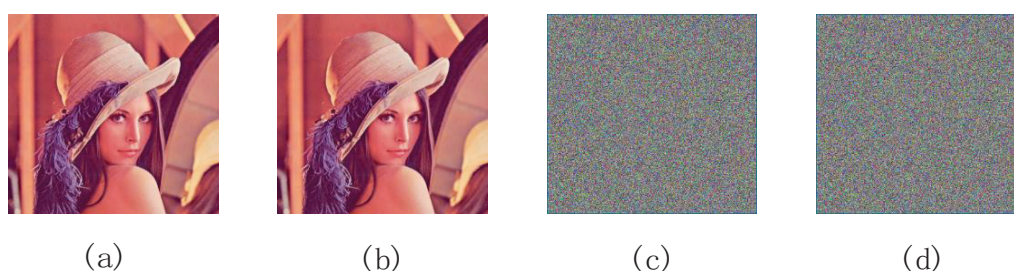
Figure 12. Key sensitivity test. (a) Plaintext image, (b) Decryption image \tau_A = 0.1521 , (c) Decryption image \tau_A = 0.1522 , (d) Decryption image d_x = 400 .
