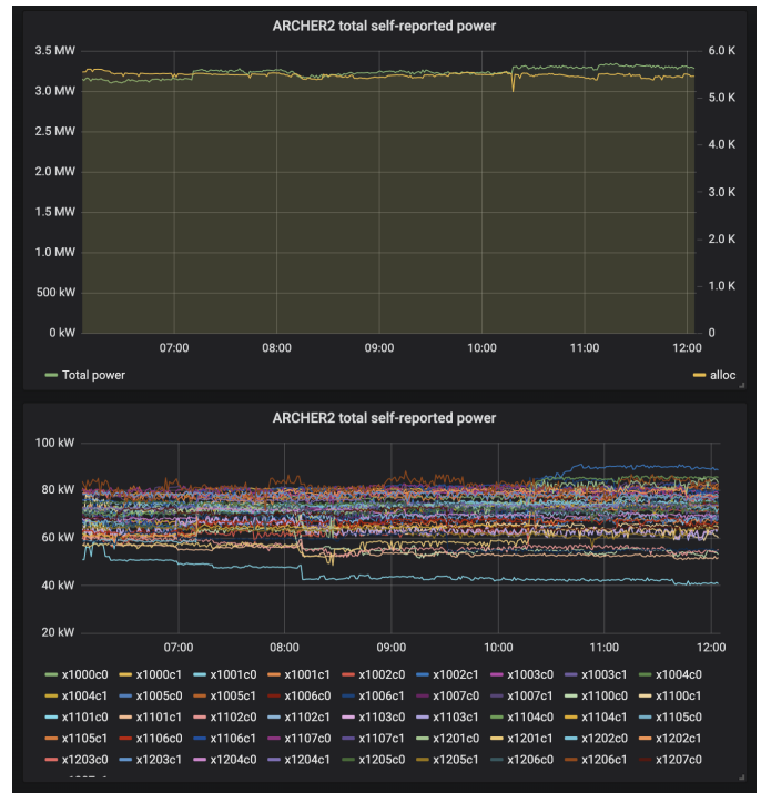
Fig. 4. Graphs showing the whole system and per-cabinet power data gathered
