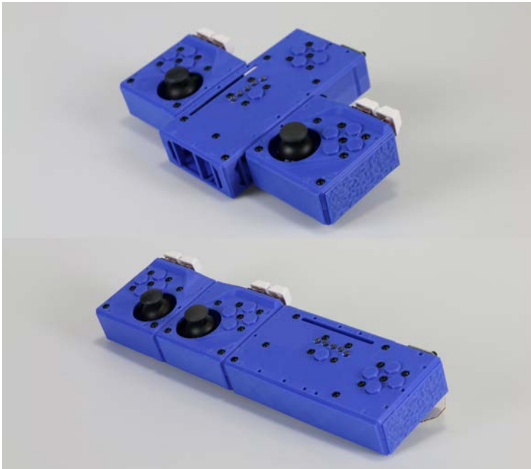
Fig. 5 Gamelon Pad. The complete device with “T” and linear shape setup. Photo, by N. Scalzotto.
