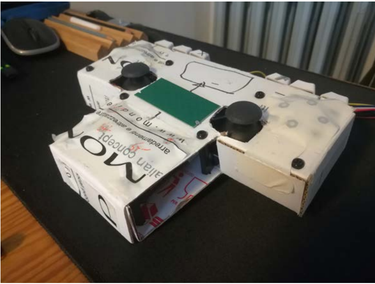
Fig. 3 Gamelon Pad. The first mock-up used for UX (User Experience) testing. Photo, by N. Scalzotto.
