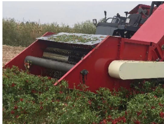
Figure 9. Field test of the prototype picking machine.
