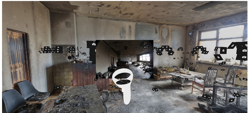
Fig. 4 First-person view of the site reconstructed using photogrammetry. Images produced in the photogrammetric acquisition are displayed as interactable floating images
