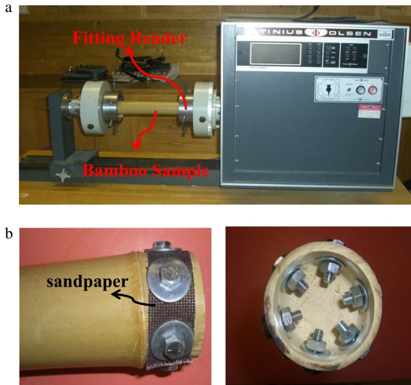
Fig. 1. (a) Experimental setup. (b) Fixtures (grit drywall sandpaper, bolts and matching nuts) that were used to secure the bamboo sample during the torsion test.
