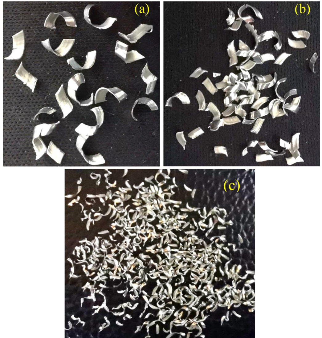
Fig 2. Aluminum machined chips; (a) large, (b) medium and (c) small size.
