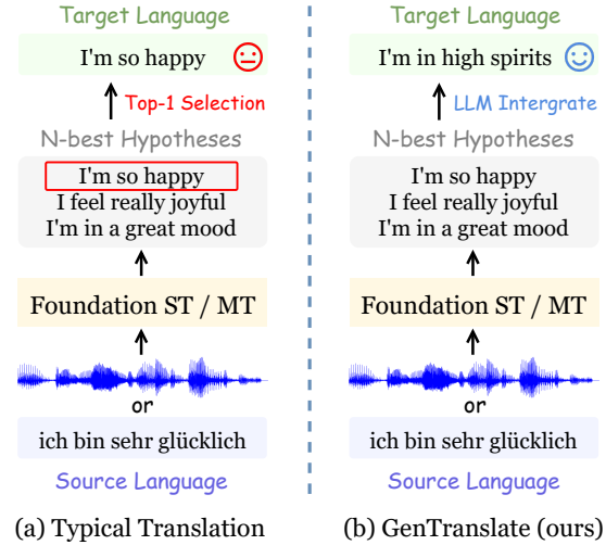
Figure 1: Illustration of (a) Typical seq2seq translation with beam search decoding and top-1 hypothesis selection, (b) our “GenTranslate” with LLM integration.
