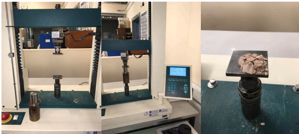
(a) (b) (c) Fig. 7. Compression test of cylinder lined with scale; before (a), during (b) and after (c) test.
