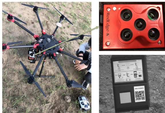
Fig. 2. UAV-Camera system: DJI S1000 UAV (left), RedEdge camera (upper-right corner) and reflectance panel (lower-right corner).
