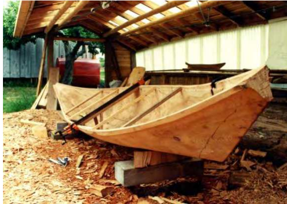
Fig. 8. Julia canoe properly steamed and spread and being finished before launching.
