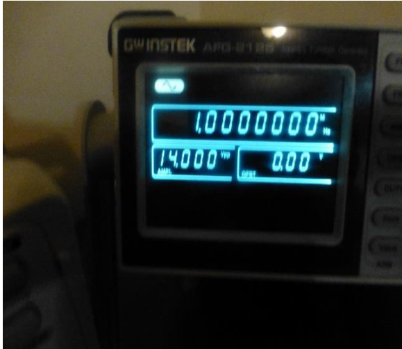
Function generator the frequency is 1 MHz and amplitude equal to 14 Vpp.
