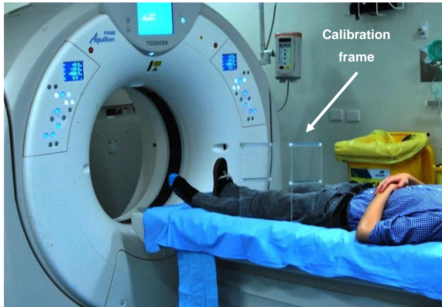
Figure 36 The Toshiba Aquilion 16 spiral CT scanner, a participant with the calibration frame over the examined knee.
