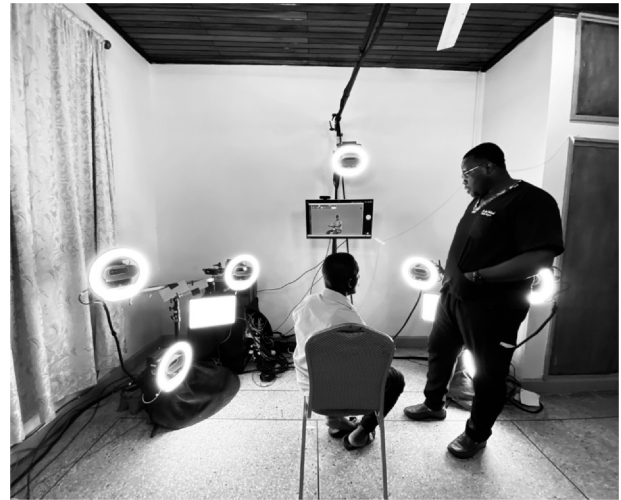
Figure 1 The Holoportation 3D Telemedicine clinic in Korle Bu Teaching Hospital, Ghana. A patient with ameloblastoma of the mandible talks with Levi Ankrah, Consultant Plastic Surgeon. They are surrounded by 10 Kinect cameras, and the patient can view the 3D images on the screen in front of them.
