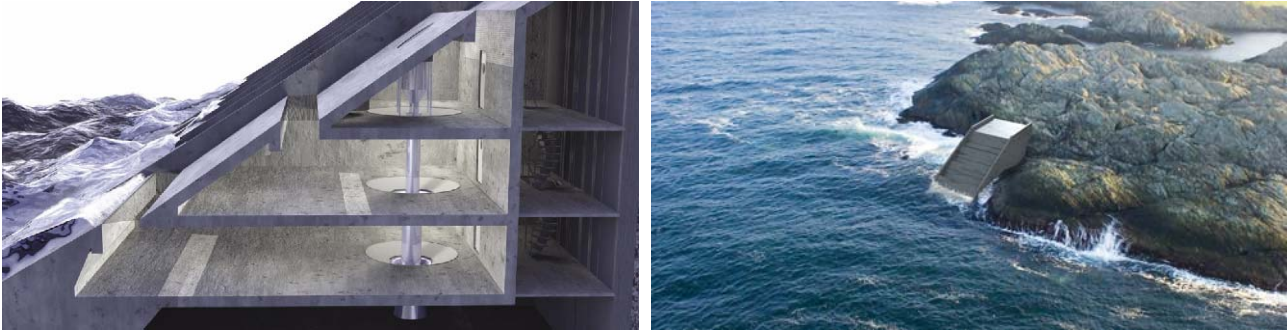
Fig. 6: Illustration of the Seawave Slot-cone as an integrated part of a breakwater (left). Photo montage of pilot plant to be installed on the west coast at the island of Kvitsøy, near Stavanger, Norway (right).
