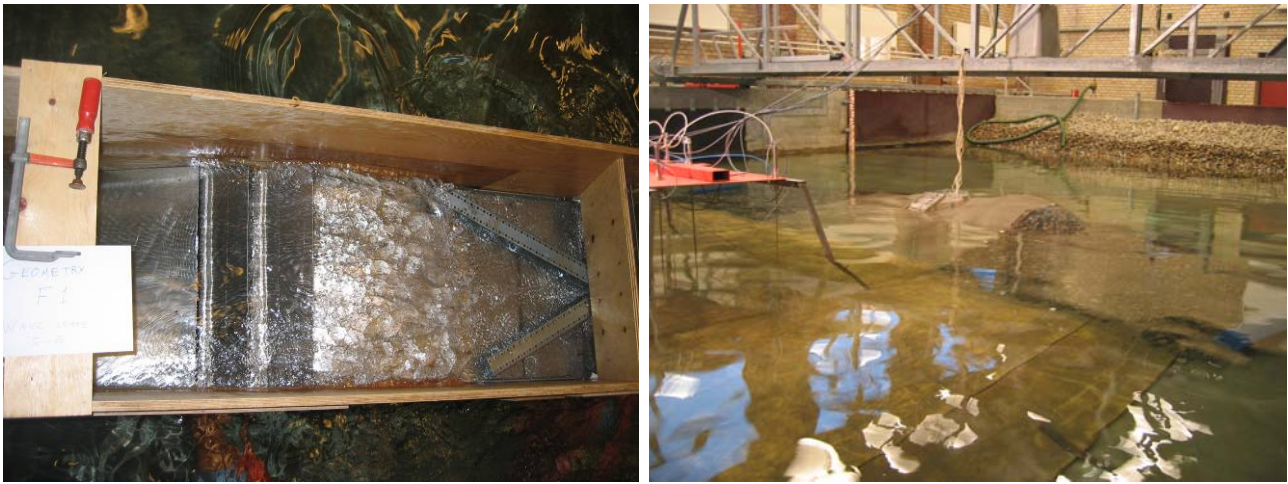
Fig. 7: Performance optimization of geometric layout through wave tank model tests (left). 3D performance model testing in wave tank with model (right).
