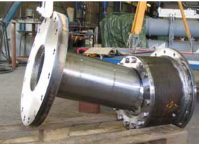
Figure 10: Manufactured joint and fitting on main platform.
