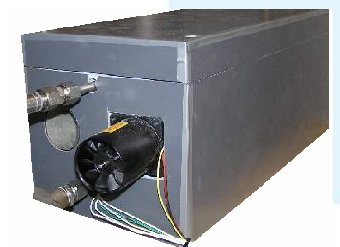
Figure 9: Picture of fuel cell stack in insulated box with axial blower mounted on the outside.
